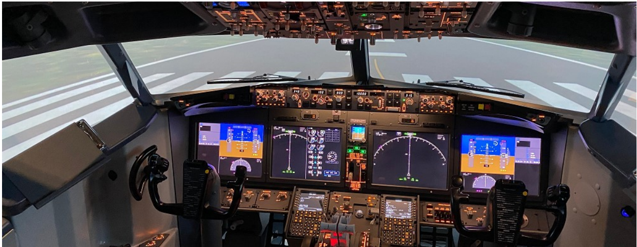
Showing Sim-Avionics software running in a FlightDeckSolutions 737Max Flight Training Device
